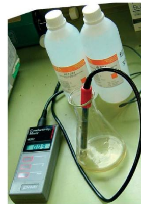
Figure 2: The conductivity of the filtrate is measured using a calibrated conductivity meter using a dip cell
