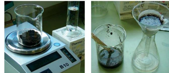
Figure 1a and b: 20 g of media are mixed with 100 ml of water, which is used for germination tests 1 , at 20°C ± 1°C (a). This is mixed and left for 30 min before filtering (b).
