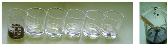
Figure 1a and b: For sand and organic growing media, one volume of media is mixi with 5 volumes of water that is to be used for germination tests. The mixture is stirri for 5 min and then allowed to stand for a minimum of 2 hours and a maximum of ; hours. After standing the mixture is stirred and the stabilised pH value of the suspensi solution measured.
