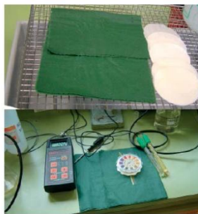
Figure 2a and b: Paper media samples are moistened with water that is to be used for germination tests 1 and the pH is measured on the surface of the paper. The pH is measured using a calibrated pH meter or pH paper.
