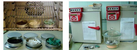
Figure 1a and b: The Moisture Content of the Germination media is measured using the ISTA Constant Temperature Oven method at 130°C.
