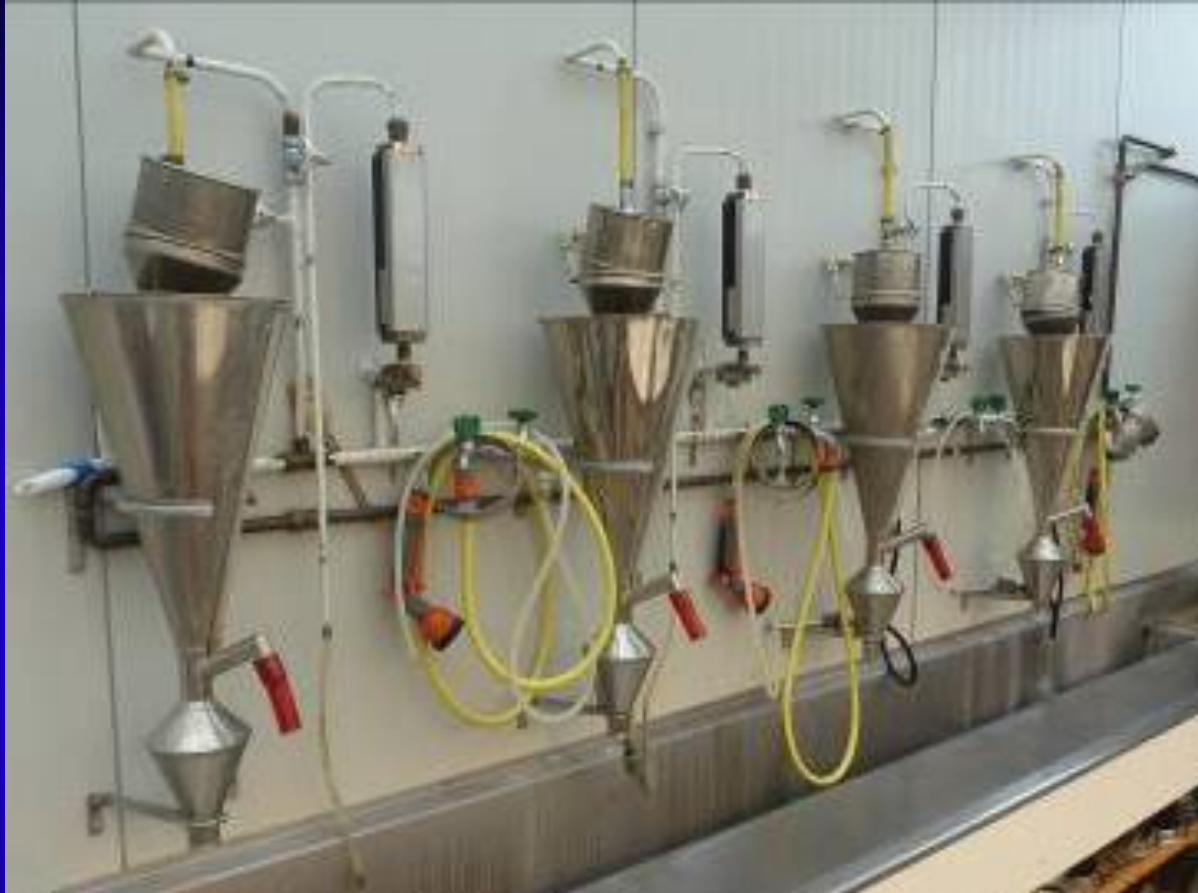
Standard Oostenbrink elutriator made of stainless steel (EPPO Website)
