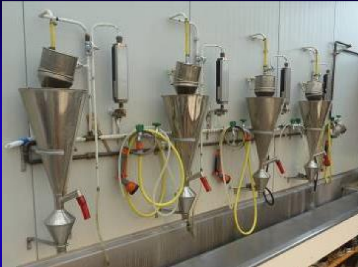
Standard Oostenbrink elutriator made of stainless steel (phot. EPPO Website)
